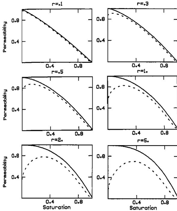
Figure 2. Permeability of medium with tapered cracks using corrected (solid line) and original (dotted line) Kozeny-Carman equations. Permeability was normalized by its value at  $Z = 0$ .
