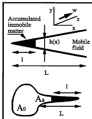
Figure 1. Thin tapered pore and pore with tapered appendix with accumulated immobile matter.
