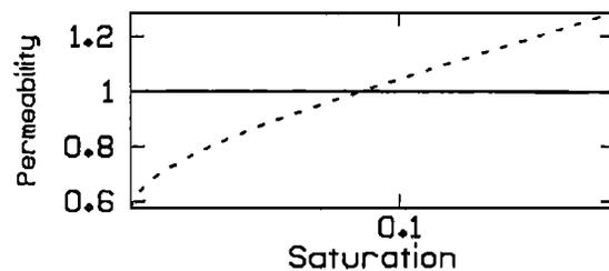
Figure 4. Relative permeability of a medium with circular pores and two thin triangular appendices using corrected (solid line) and original (dotted line) Kozeny-Carman equations. Permeability was normalized by its value at  $Z = 0$ .
