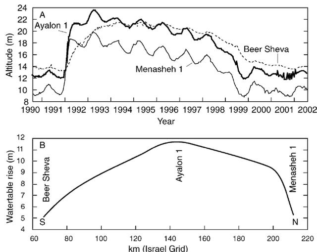
Fig. 10. Yarkon–Taninim aquifer water levels (data from the Israel Hydrological Service): (A) A 12-year-long level record of three observation wells from the north (Menasheh 1), center (Ayalon 1) and south (Beer Sheva) parts of the aquifer. (B) Relative change of water level from November 1991 to April 1993 along a north–south transect.
