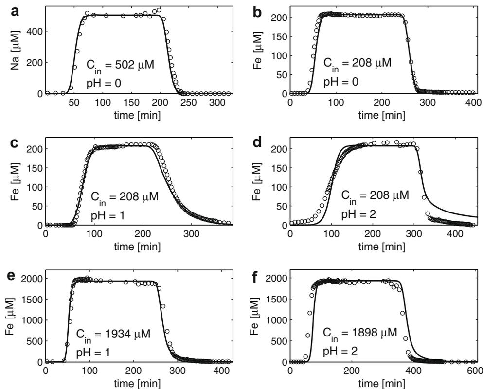
Fig. 4. Experimental breakthrough data for (a) Na and (b–f) Fe solutions. Inlet concentrations ( $C_{in}$ ) and pH are indicated for each experiment. Summary of experimental conditions is given in Table 1. Solid lines indicate the model breakthrough curves.
