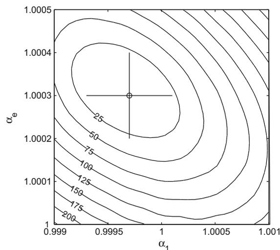
Fig. 6. Error map for different values of  $\alpha_1$  and  $\alpha_e$ . The error is given as a percent increase relative to the minimum value (indicated by the circle) at  $\alpha_1 = 0.9997$  and  $\alpha_e = 1.0003$ . Note that the error function is relatively smooth, converging in the region bounded by the 25% error contour, which serves as a basis for the estimated error bars. The contour lines were interpolated from over 300 points using a Delaunay triangulation method.
