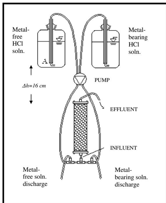
Fig. 3. Experimental apparatus. The diagram illustrates the scheme for the sequential introduction of the metal-bearing and metal-free HCl solutions from two glass Mariott bottles (shown at top).
