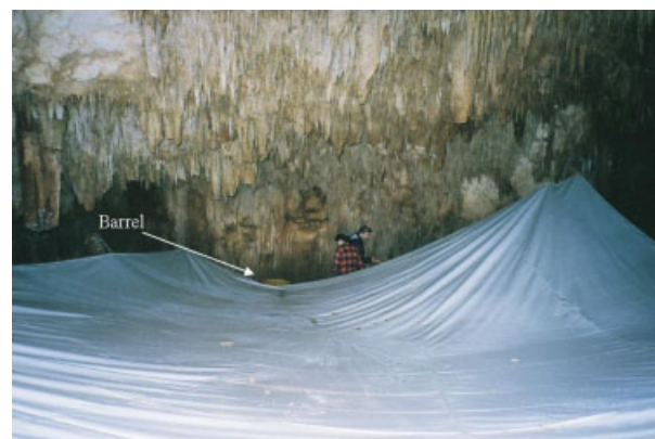
Figure 3. The collection sheet at Site 2, funnelling the drip water into a barrel at the far end of the sheet. This barrel is equipped with a pressure transducer connected to a 5 min interval data-logger, recording the water level in the barrel. Note the ceiling, densely decorated by speleothems
