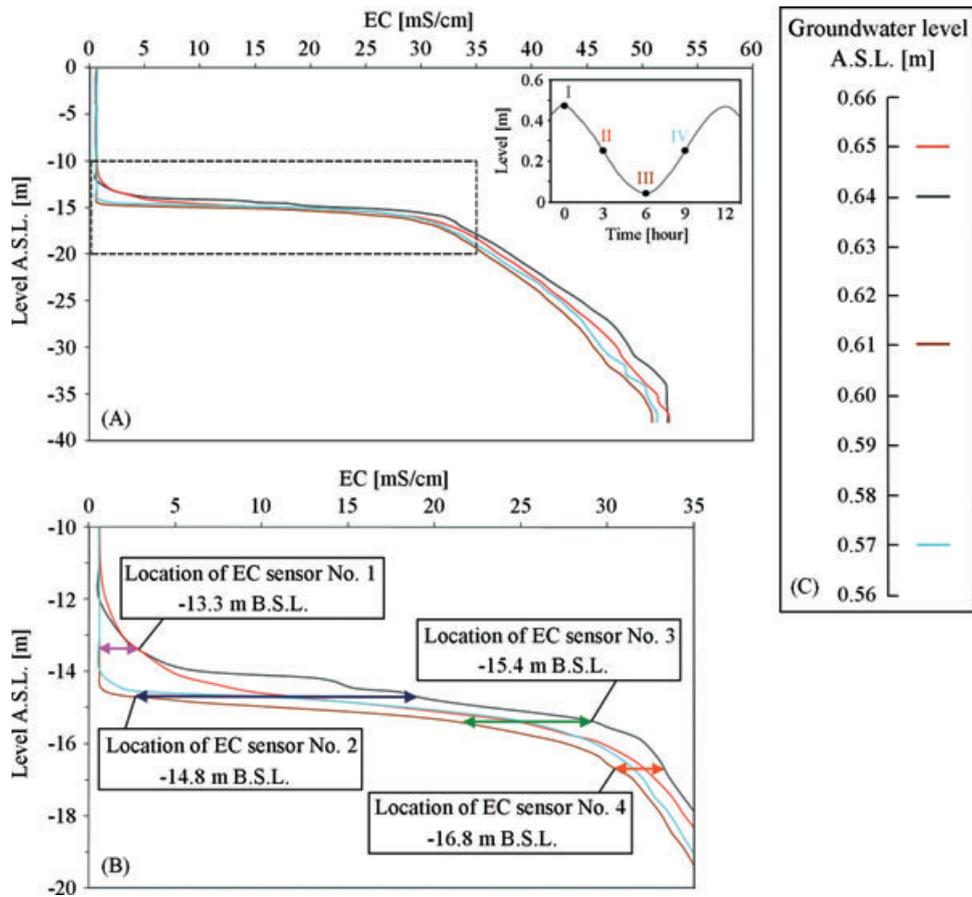
**Figure 5.** EC profiles and groundwater level in borehole LP-3 (long-perforated) on four stages of daily tide cycle on 28/8: I – High tide; II – Mid-tide on ebb; III – Low tide; and IV – Mid tide at sea rise. Zoom-in of the broken frame is presented in the lower part of the figure.
