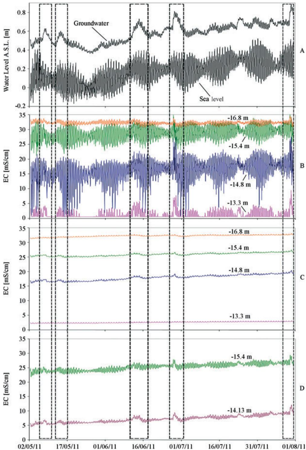
**Figure 4. Top to bottom: (A) Sea level and groundwater level in LP-3; (B) EC in four sensors located at different depths in long-perforated borehole LP-3; (C) EC in four sensors buried at the same depths in B-1; and (D) EC in two sensors located at different depths in short-perforated boreholes SP-1 and SP-2. The broken frames represent events with a sharp rise in groundwater level due to stormy sea. Numbers on B, C, and D represent the depths of the sensors.**
