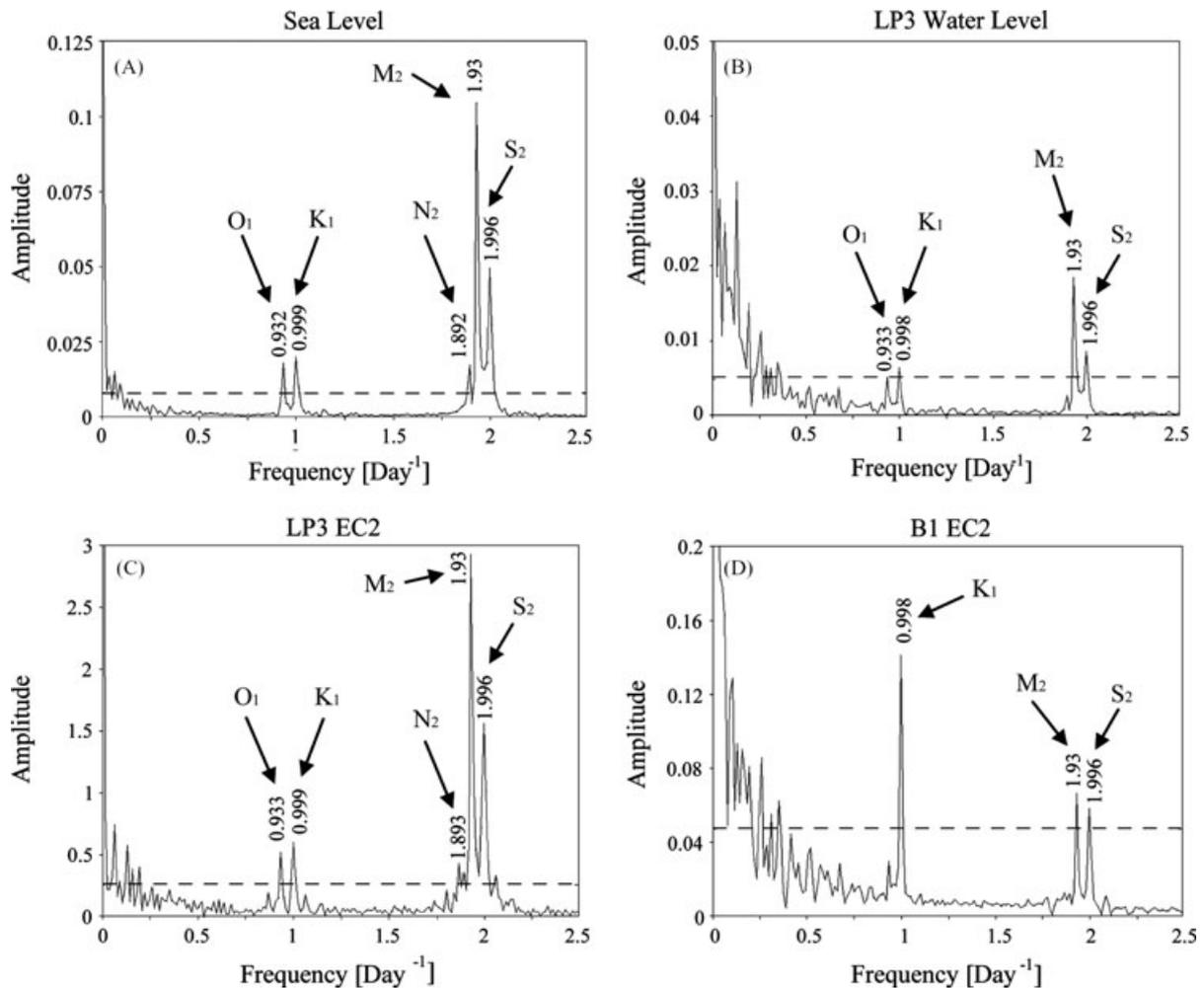
**Figure 6.** Main frequencies of sea level, groundwater level and sensor EC2 from the LP-3 borehole (long-perforated) and sensor EC2 from the buried sensor in B1, as obtained by Fast-Fourier-Transform (FFT) analysis. The broken line represents a significance of 95%. Low frequencies (0 to 0.5 d<sup>-1</sup>) include a lot of noise due to the relatively short duration of measurement. Note that the amplitude axes on the different graphs are not on the same scale.
