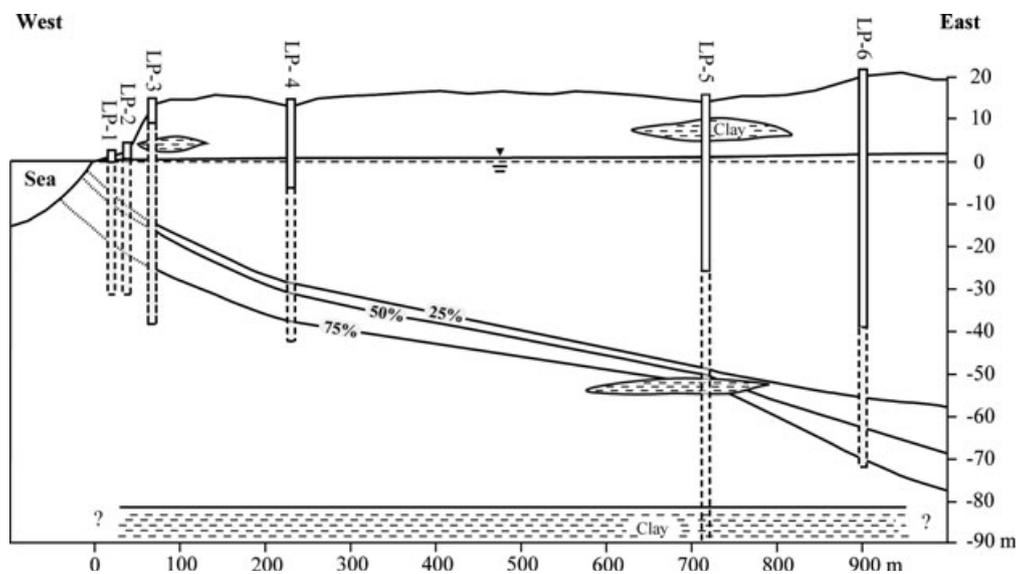
**Figure 3.** Cross section of the transition zone between fresh and saline waters perpendicular to the shoreline in the research area. Groundwater salinity isopleths are marked by black lines. The broken lines in the boreholes represent the perforated segment. On the vicinity of the shoreline the location of the transition zone was estimated because the groundwater is consistently affected by sea waves.
