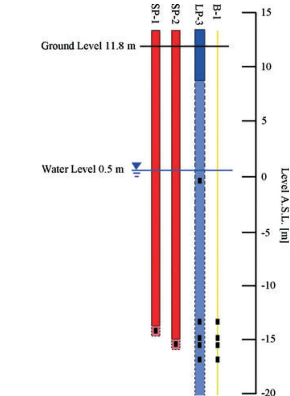
Figure 2. Location of sensors in LP-3, SP-1, SP-2 and B-1, all located 70 m from shoreline. The broken line represents the perforated segment of the borehole. Note that borehole LP-3 is deeper than shown in this figure.
